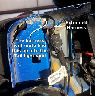
Once there, remove the passenger side tail light. This can be accessed from the right rear interior corner. There is a small plastic cover. Carefully remove this cover with the appropriate panel tool.
